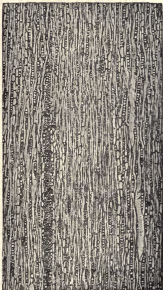
FIG. 27.—Tangential longitudinal section of oak wood, magnified fifty diameters, and showing the transverse sections of the medullary rays, cut as they project towards the observer. (Müller.)
